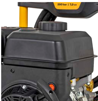
Fuel tank The engine is designed to run on unleaded 95 petrol. Never use contaminated fuel or an oil and petrol mixture. Avoid dirt or water in the fuel tank. To check the fuel level and fill the tank, the engine must be stopped.
