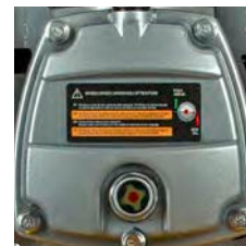
Oil level sight glass
