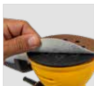
Velcro-type fastening of the sanding sheets
