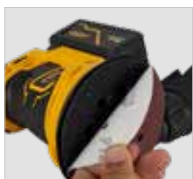
Velcro-type fastening of the sanding sheets
