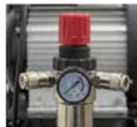
Outlet valves with pressure regulator
