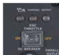
ESC switch (electronic speed control)
